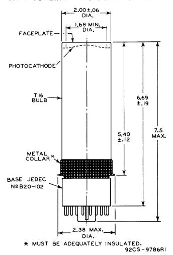
$\mathbb{C}$  of bulb will not deviate more than  $2^{0}$  in any direction from the perpendicular erected at the center of bottom of the base.
