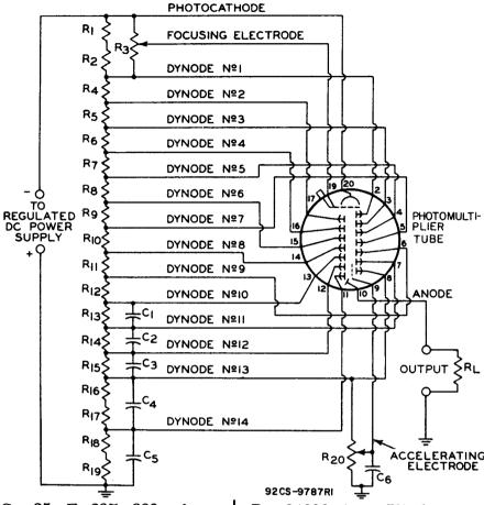
C<sub>1</sub>: 25 pF, 20%, 600 volts (dc working), ceramic disc C<sub>2</sub>: 50 pF, 20%, 600 volts (dc working), ceramic disc C<sub>3</sub>: 100 pF, 20%, 600 volts (dc working), ceramic disc C<sub>4</sub>: 250 pF, 20%, 600 volts (dc working), ceramic disc C<sub>5</sub>: 500 pF, 20%, 600 volts (dc working), ceramic disc C<sub>6</sub>: 100 pF, 20%, 1000 volts (dc working), ceramic disc C<sub>6</sub>: 100 pF, 20%, 1000 volts (dc working), ceramic disc
