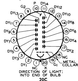
Metal Collar: Connected Internally to Focusing Electrode - Do Not Make Electrical Connection to Collar.
