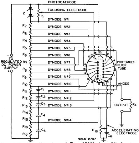
C<sub>1</sub>: 25 pF, 20%, 600 volts (dc working), ceramic disc C<sub>2</sub>: 50 pF, 20%, 600 volts (dc working), ceramic disc C<sub>3</sub>: 100 pF, 20%, 600 volts (dc working), ceramic disc C<sub>4</sub>: 250 pF, 20%, 600 volts (dc working), ceramic disc C<sub>5</sub>: 500 pF, 20%, 600 volts (dc working), ceramic disc C<sub>6</sub>: 100 pF, 20%, 1000 volts (dc working), ceramic disc R<sub>1</sub>: 5 megohms, 20%, 1/2 watt, adjustable  $R_2$  through  $R_{11}$ : 22000 ohms, 5%, 1 watt
